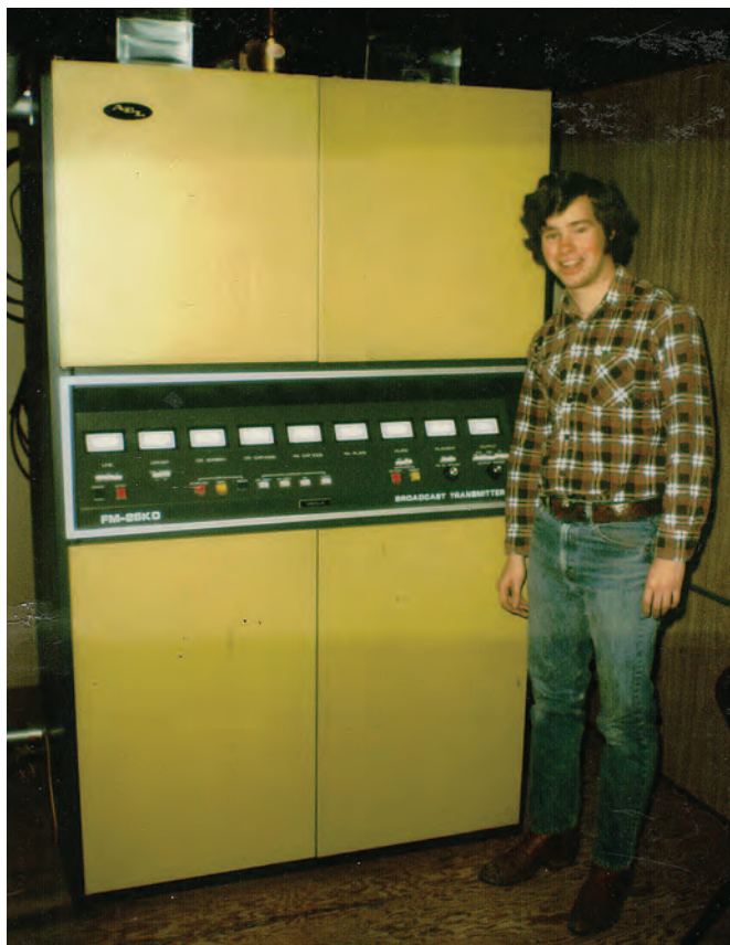
A 21-year-old Davis with the big AEL FM25KD and its even bigger power supply problems.
